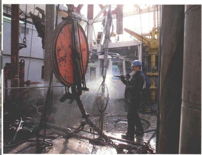
Technician washes well logging probe that has just been removed from well or "hole." On the floor to his right is the rotary table, which imparts rotary motion to the whole drill assembly. Well logging is an electronic technique to determine the potential of the drill location.
