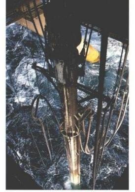
The drill stem enters water and penetrates the bottom of the sea floor. Inside the exterior conductor pipe is the surface casing and drill pipe leading down to the drill bit itself, chewing through layers of rock.
