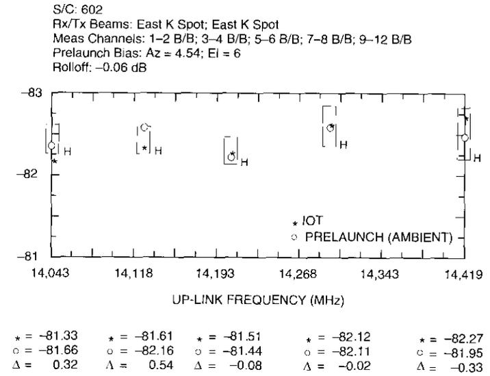
Figure 7. Typical Flux Density Graphical Test Results
