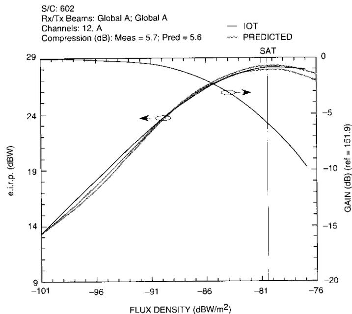
Figure 4. Example of Spacecraft TWTA Gain Transfer Characteristics Data
