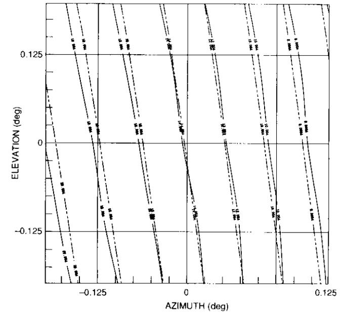
(b) 602 Rx BTS Az Modulation Index In-Orbit to Near-Field Comparison
