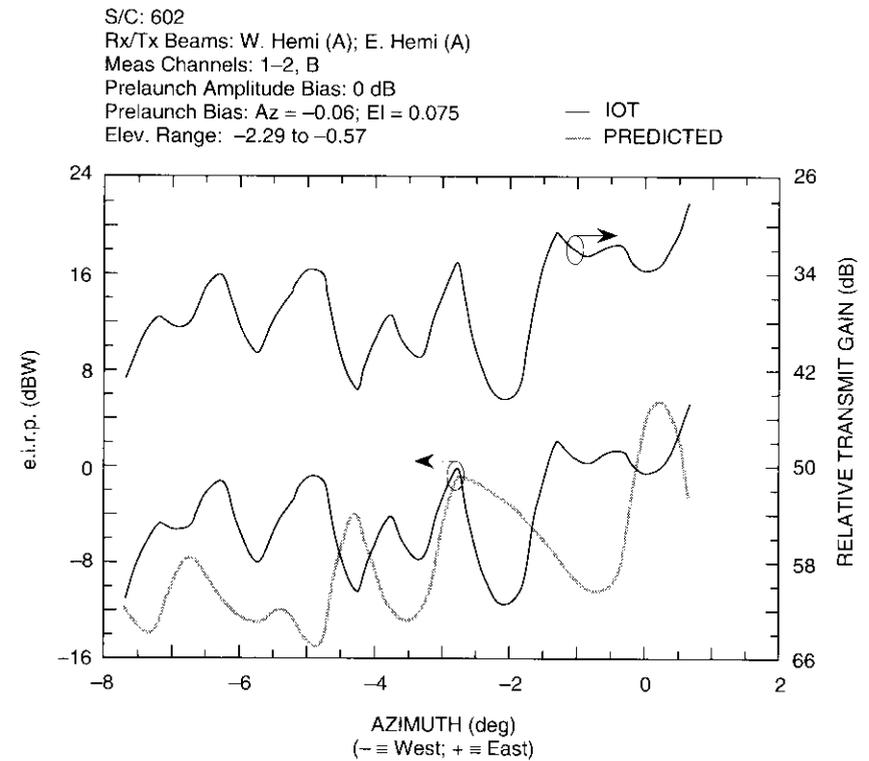
Figure 23. Transmit Sidelobe Graphical Test Result
