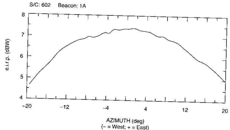
Figure 25. Example of Beacon Co-Polarized Antenna Pattern IOT Result
