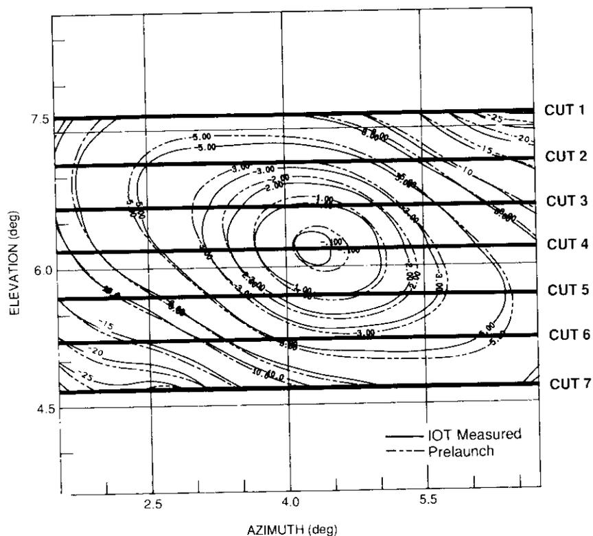
Figure 29. INTELSAT VI East Spot Beam Contours
