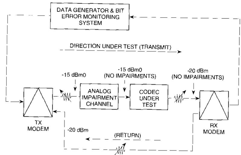
Figure 1. Voiceband Data Modem Test Configuration
