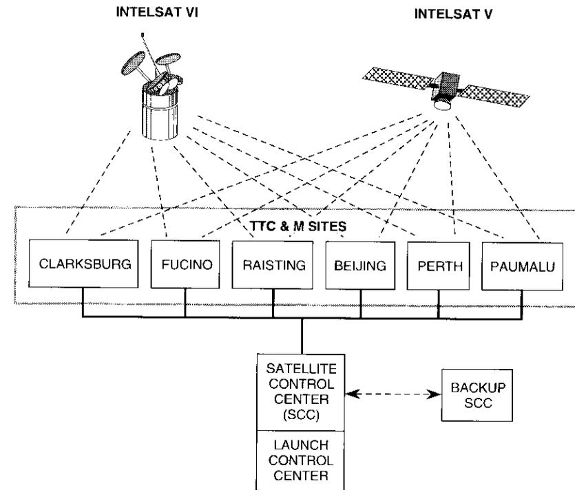
Figure 1. *INTELSAT ISCC and TTC&M Sites*
