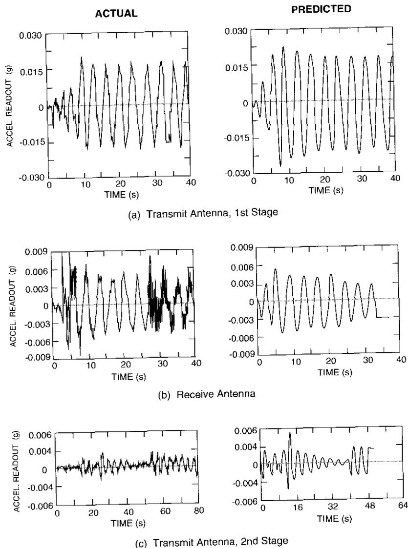
Figure 8. *INTELSAT 602 C-Band Antenna Deployment: Actual vs Predicted Accelerometer Signatures*
