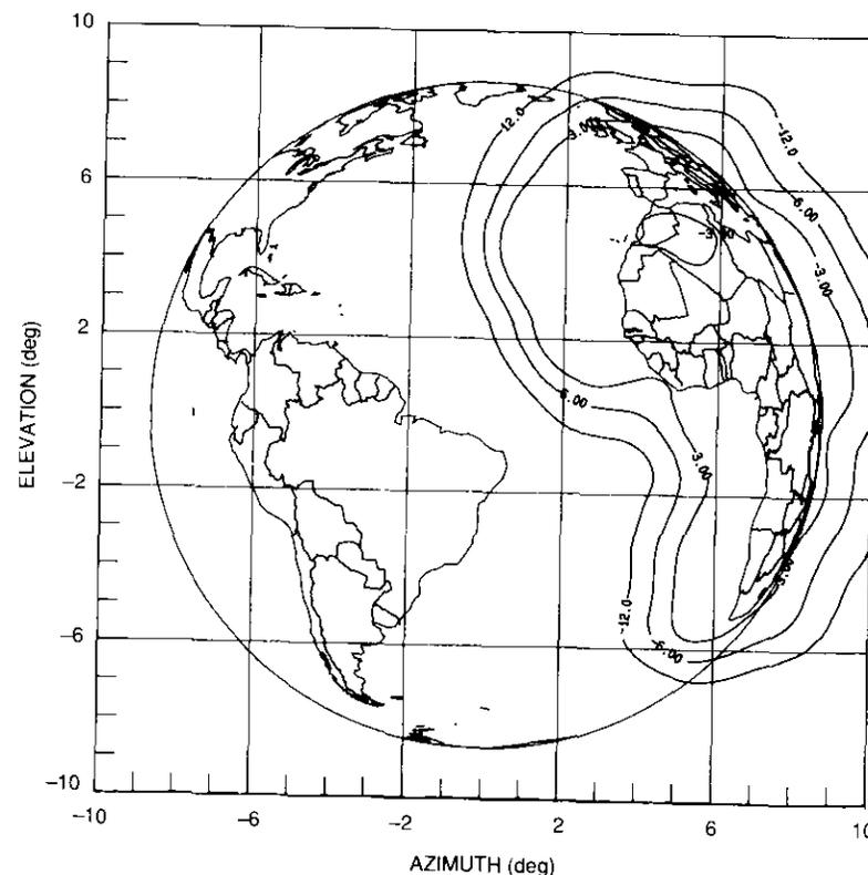
Figure 15. Typical East Hemi Beam-Pointing During IOT Tests
