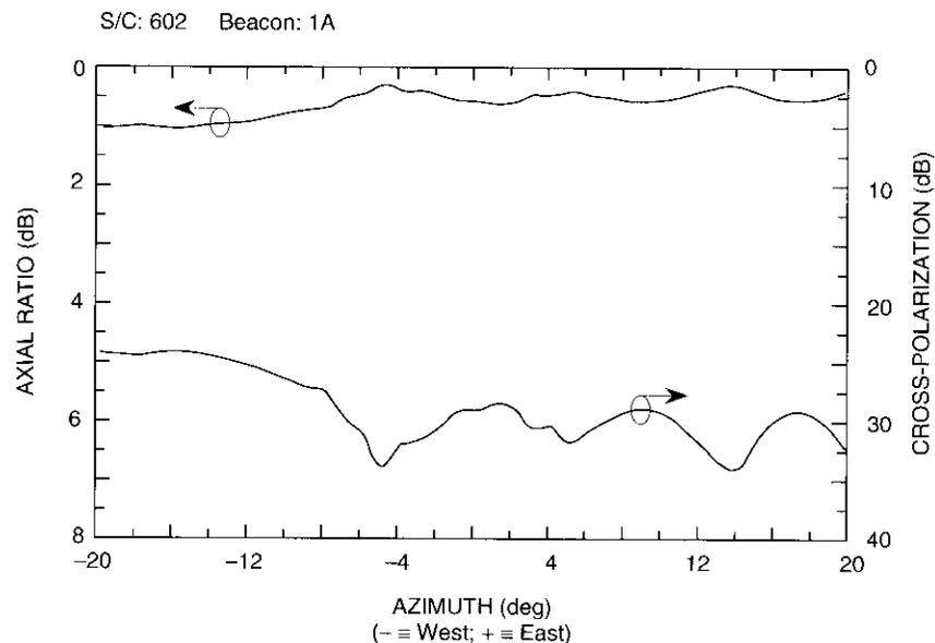
Figure 26. Example of Beacon Cross-Polarized Antenna IOT Result
