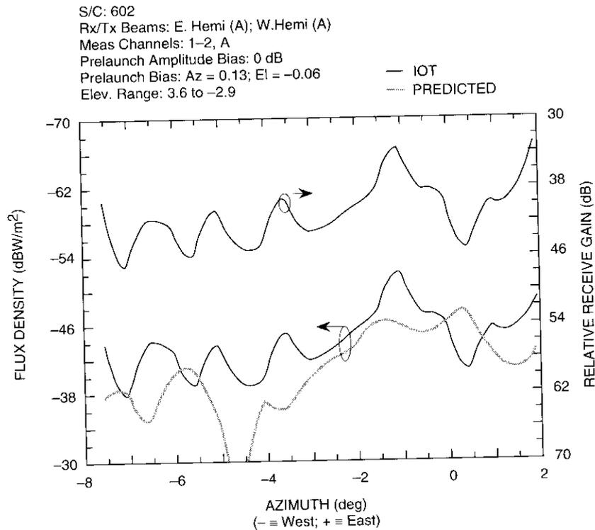
Figure 22. Receive Sidelobe Graphical Test Result
