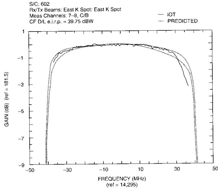
Figure 10. Example of In-Band Frequency Response Results
