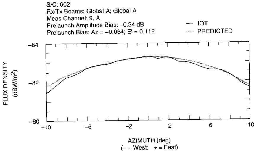
Figure 18. Example of Co-Polarized Receive Antenna Pattern Graphical Result
