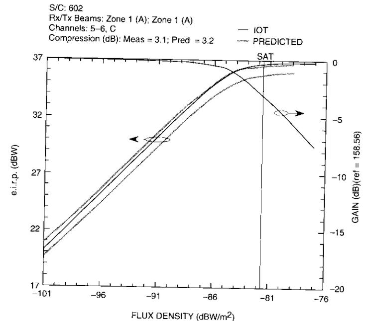
Figure 5. Example of Spacecraft SSPA Gain Transfer Characteristics Data
