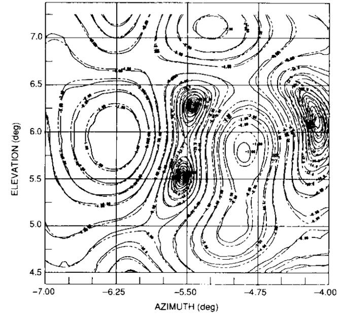
(a) 604 Rx BTS Az Channel Far-Field to Near-Field Comparison
