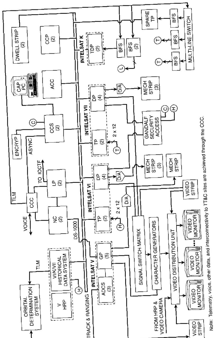
Figure 5. INTELSAT V/VI TTC&M Data Processing Network
