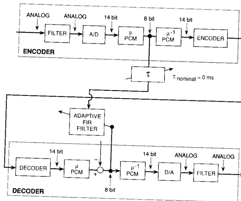
Figure 5. Measurement of Codec Delay
