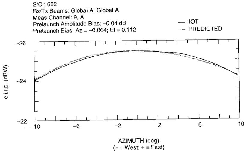
Figure 19. Example of Co-Polarized Transmit Antenna Pattern Graphical Result
