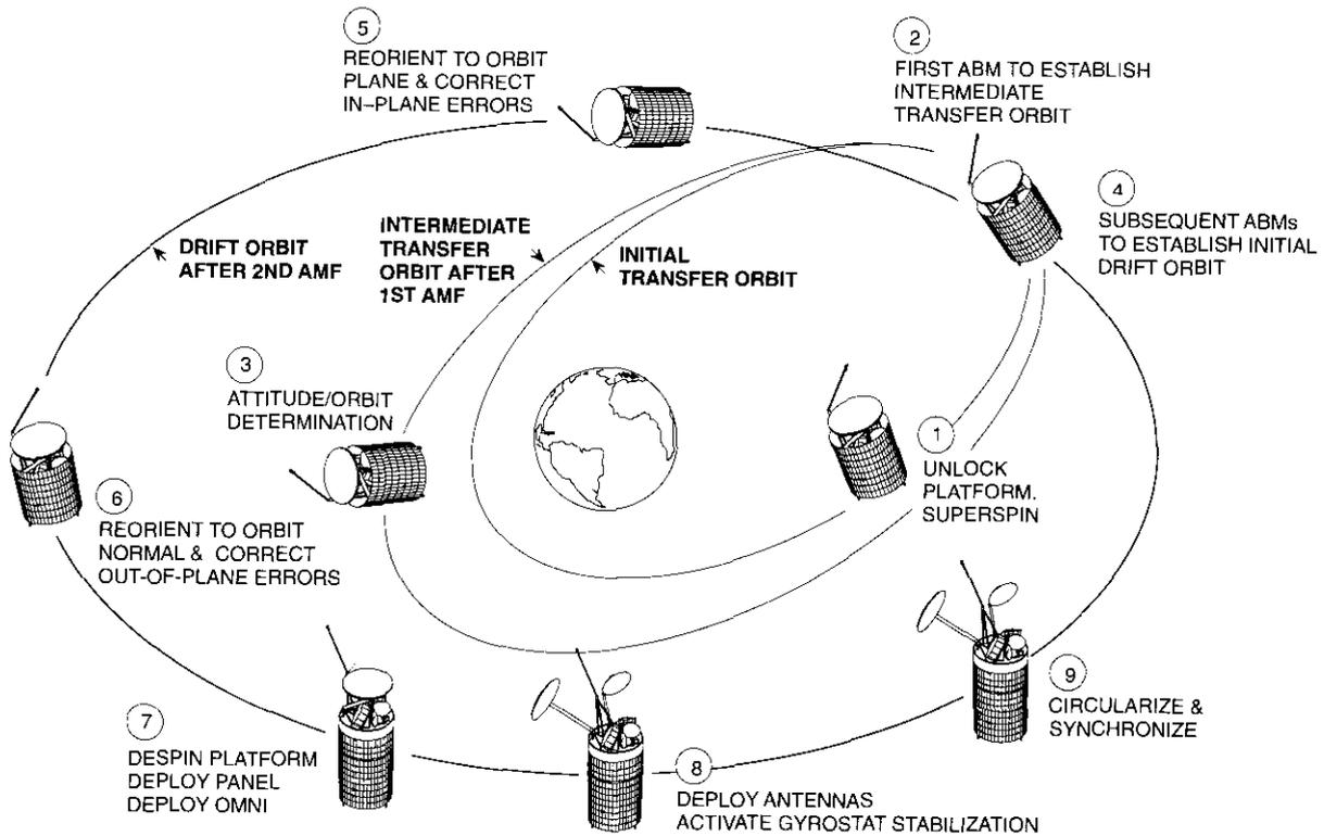
Figure 2. *Synchronous Orbit Acquisition*
