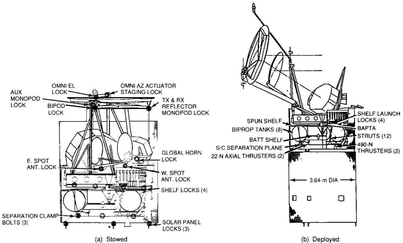
Figure 4. INTELSAT VI Antenna Configurations
