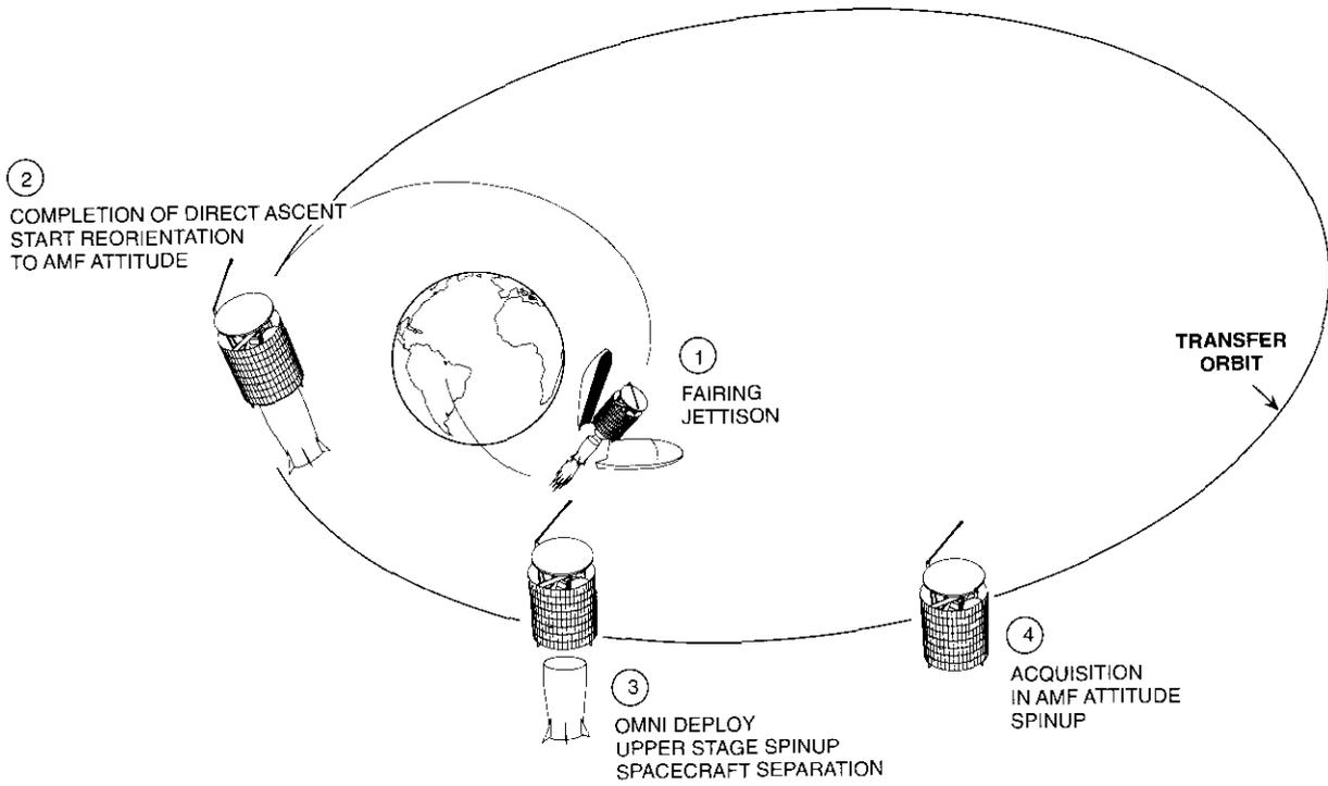
Figure 1. *Transfer Orbit Injection*
