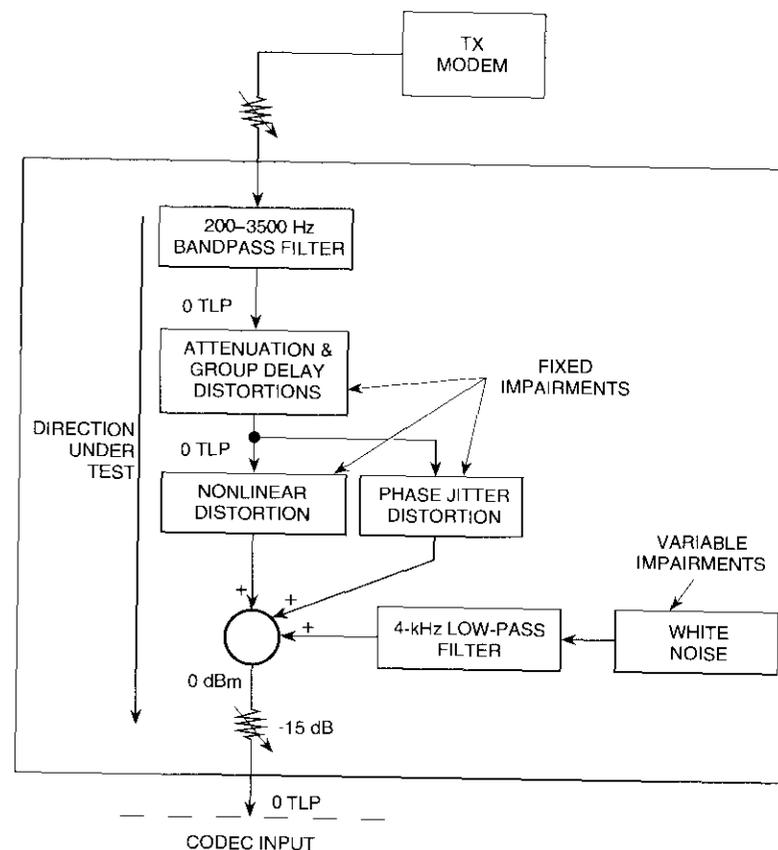
Figure 2. Configuration of the Analog Impairment Channel
