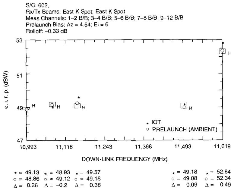
Figure 8. Typical e.i.r.p. Graphical Test Results
