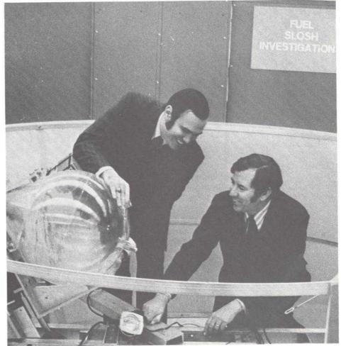
Ernesto R. Martin, principal COMSAT investigator for the project, and James R. Owens, manager of the positioning and orientation branch, COMSAT Labs, with the spinning device used to simulate the sloshing of fuel on INTELSAT IV.
