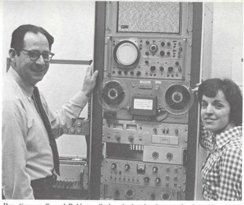
Drs. Campanella and Robinson display the baseband processing branch's analog-digital/digital-analog data link. The device converts analog signals like speech or television to digital form for Fast Fourier Transform (FFT) computer analysis. It can also "play back" by reconverting digital data to analog signals for subjective evaluation.
