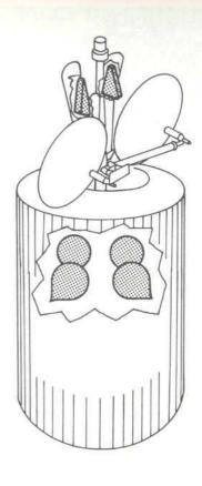
A simplified drawing of INTELSAT IV showing the four fuel tanks in the spinning drum and the two nutation dampers on the despun platform.
