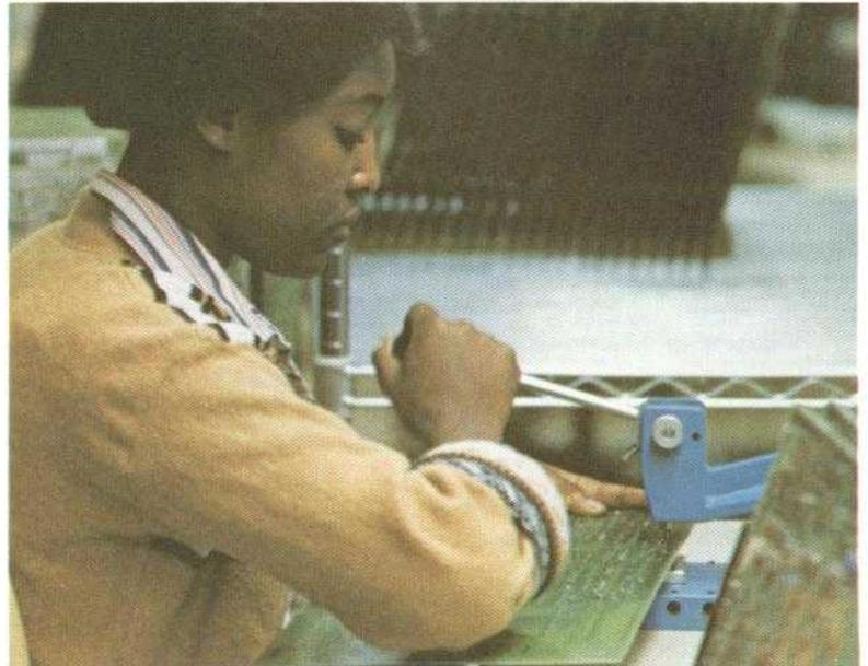
*Darlene Blake hand-operates a device that inserts test point terminals into PC boards.*
